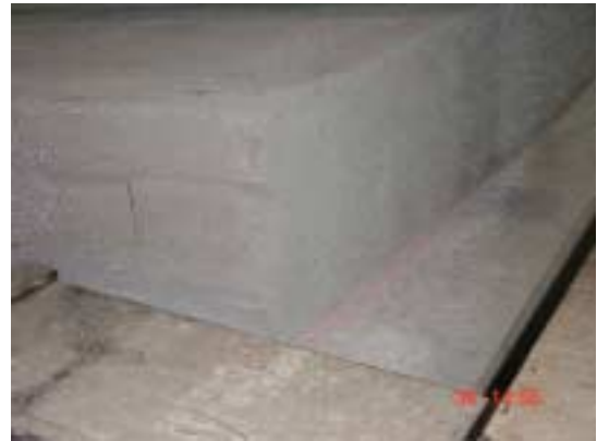
Sandwich slab Phase 2 at 70 minutes. Deflection and support.
